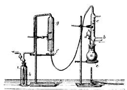
sample are put into a crucible, which is then placed into the 500 c.c. flask, a. A current of hydrogen is passed through the tube b, and when the air has been expelled the burner, f, is lit and the pump, attached to the exit tube of the wash-bottle h, put intoAfter fitting on the condenser, 30 c.c. of absolute alcohol are introduced drop by drop
